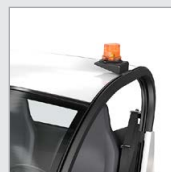
SECURITY LIGHT BEACON
