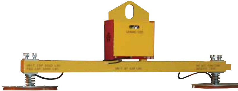
Custom designed bail for large crane hook.
